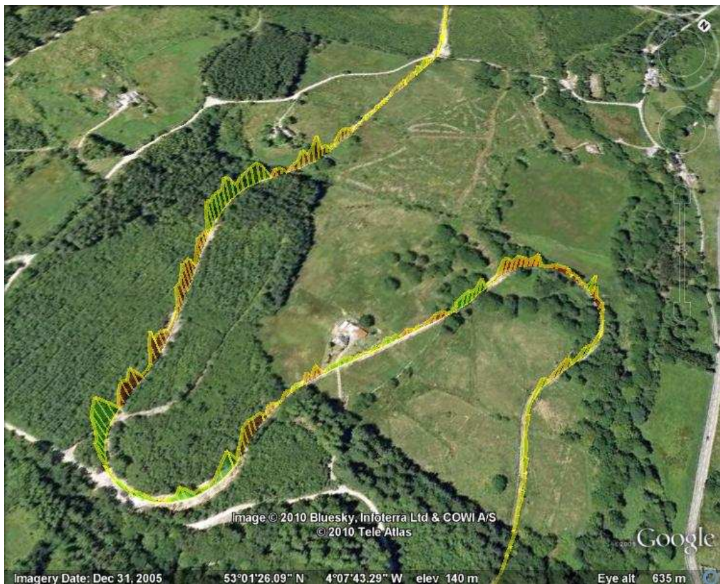
Figure 8. Rhyd Ddu to Beddgelert — x as height — high-pass filter, \sigma = 15 bins
